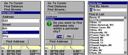
Find City field (left). Search in particular city only option (center). Find City by name (right). 6. When the necessary search fields are filled in, press  $\downarrow$  to FIND ADDRESS | ENT. Your unit asks you to wait while it searches for the address. (If an address is not in the database, a message appears saying the address could not be found.)
